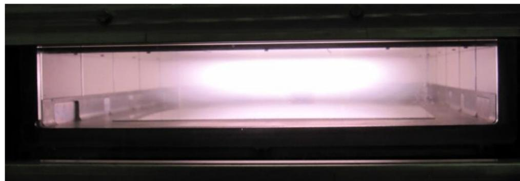
Example of a large area plasma reactor 1 m x 1 m
